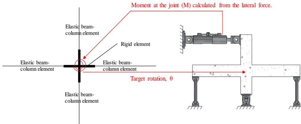
Fig. 1 Hybrid simulation method using the lumped spring
