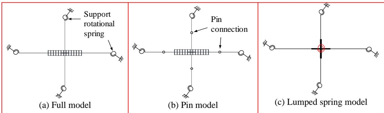
Fig. 3 Analytical models for the parametric study ( $K_s = 10^8, 10^9, 10^{10} \text{ N}\cdot\text{mm}/\text{rad}$ )
