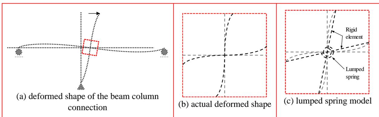
Fig. 2 Representation of the deformation with the lumped spring and rigid elements
